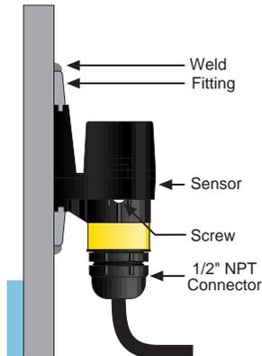
2. Determine the mounting location for the level switch. The point of actuation (where the sensor will send a "wet" signal) is most often at the center of the sensor; however the actual Point of Actuation (POA) may differ depending on the application liquid and tank wall characteristics. After positioning the fitting to check clearances, etc., remove the paper protective strips from the adhesive of the fitting.
