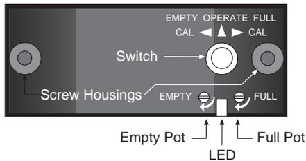
4. Empty state: With the tank drained to a point no closer than 6 inches below the bottom of the sensor, set the switch to the Empty position (left). Set the Empty trimpot as in Step 3.
